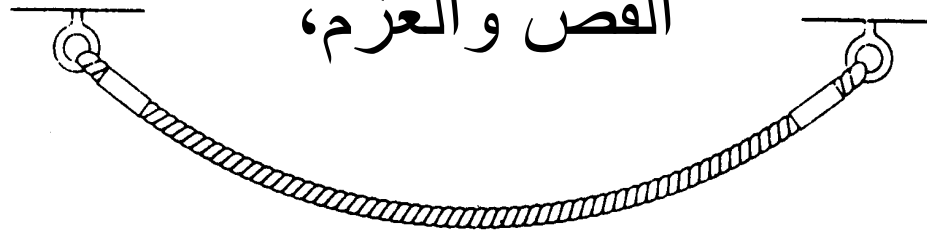
Cables support their loads in tension
